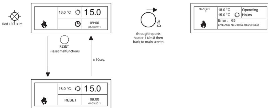
With the Reset button, the Malfunction can be rectified after which the Message will disappear and the main screen is shown again on the display.
